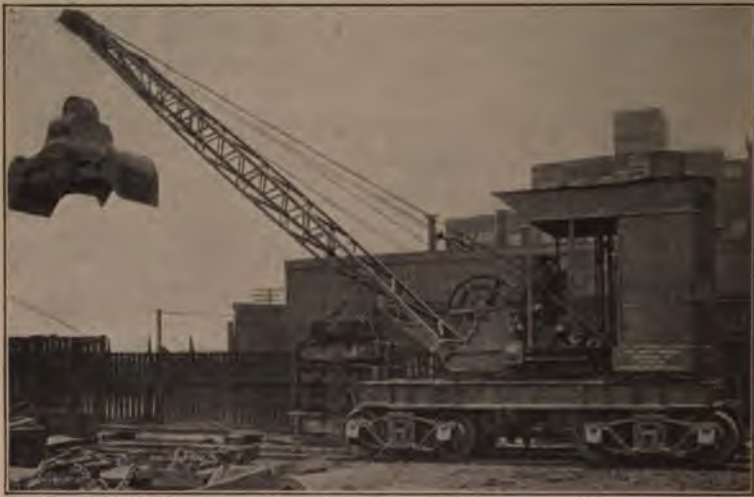
Travelling Crane Equipped with Crab Bucket.
